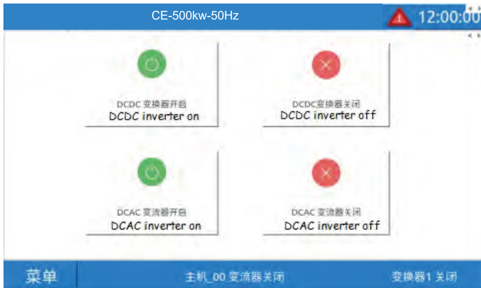
Figure 7-4 Startup and shutdown main interface
