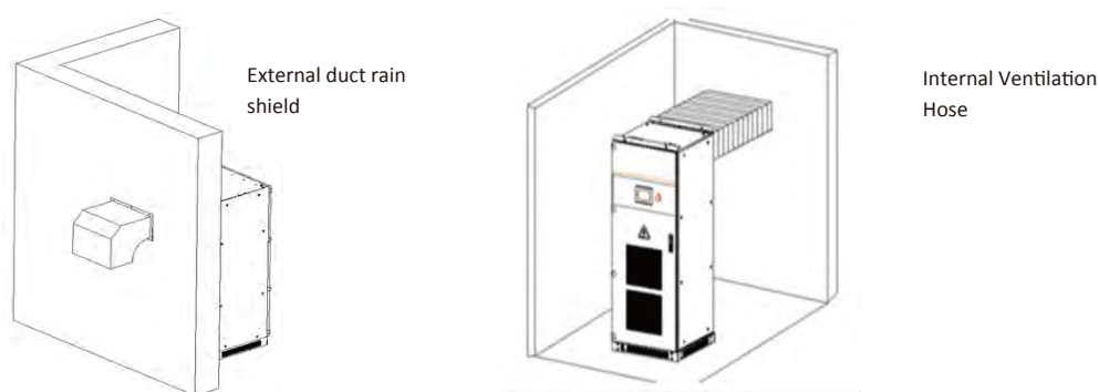
Figure 5-7 Schematic diagram of inverter external duct
